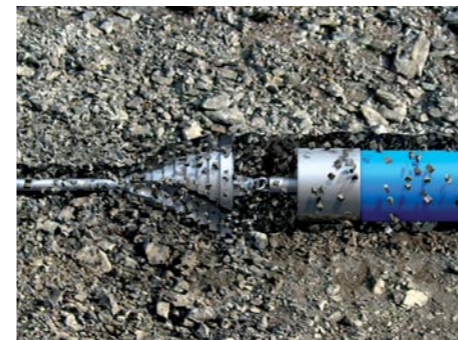
Horizontal directional drilling
