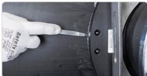
**8. Use a gap measurement gauge to check the fit of the fitting. The maximum gap is 0,3 mm\***
