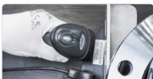
**9. Start welding, scanning the barcode placed on the fittings and proceed according to the requirements of the machine\*\***
