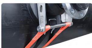
**d. Install the belts with tightener with installation roller N° 2 on the clamping tool**
