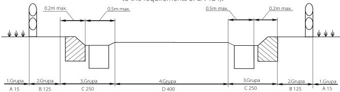
Cross section of street where different groups of chamber covers are displayed according to EN 124.
