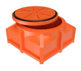
Optical cable connection chamber with waterproof cover for underground installations. Ideal for various cable systems such as optical cable lines, telecommunications lines for railway signalling systems, etc. The chamber is easy to install and the diameter of access (700 mm) provides a wide working space.
