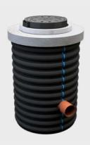
Drainage manhole with diameter of DN/ID 1000 mm and sediment trap.\* Double-wall PP height adjustment shaft with welded on base. Industrially welded connections. Reinforced concrete support ring, h=160mm. Reinforced concrete height adjustment ring, h=80mm (adjustment height 60mm, installed if necessary, no more than 4 pieces can be stacked). Stationary type cast iron cover, conform to EN 124-2, traffic load class D400(40t), opening DN/ID>600 mm.
