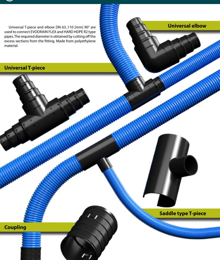
With a doublesided coupling for corrugated pipes it is easy to attach and make connections for EVODRAIN pipes. Water resistance (a pressure rating of > 0.5 bar) of joints can be achieved by additional use of the rubber sealing rings.
