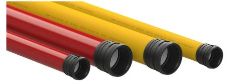
**RIGID ELECTRO** is cable protection pipe. Manufactured from polypropylene (PP) this pipe has excellent impact and load strength properties. This cable protection pipe features SEAL LOCK coupling system that includes friction welded socket and locking sealing ring ensuring watertight connections (up to 0,5 bar).
