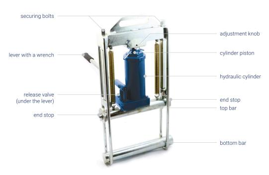
A hydraulic pipe squeeze-off tool allows you to manually / hydraulically clamp polyethylene pipes to temporarily shut off the flow of medium inside a pipeline. When using the tool, follow the health and safety rules.
