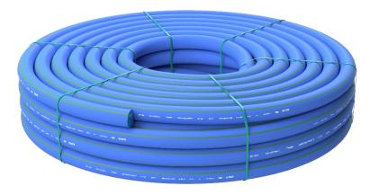
**ULTRASTRESS PROTECT** pressure pipes are made from PE100-RC material with a polypropylene (PP) protective layer (<10% of wall thickness) for additional durability. PE100-RC material pipes are resistant to long term expansion of cracks and point type loads. Point type loads are especially common during assembly of the pipelines using trenchless installation methods (for instance, as a result of friction against the stones that are
