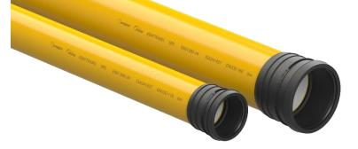
**RIGID MONO ELECTRO** is cable protection pipe, conforms Swedish standard SS 4241437. Manufactured from polypropylene (PP) this pipe has excellent impact and load strength properties. This cable protection pipe features SEAL LOCK coupling system that includes friction welded socket and locking sealing ring ensuring watertight connections (up to 0,5 bar).
