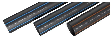
**EVOAQUA** pressure pipes for potable water (black with blue stripes) and wastewater (black with brown stripes) are made from PE80 or PE100 material. Pipes features excellent long-term durability properties, high resistance to corrosion and very low resistance to flow. Material of the pipes is chemically and biologically inert. Construction method - in open trenches with filling and bedding.
