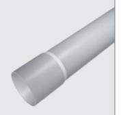
A rigid, halogen-free electrical installation conduit made of aPVC-U material grey (RAL 7037). The conduit is manufactured in straight 3 m bars, with a moulded-on coupling for quick connection. The conduit features a medium compression strength.
