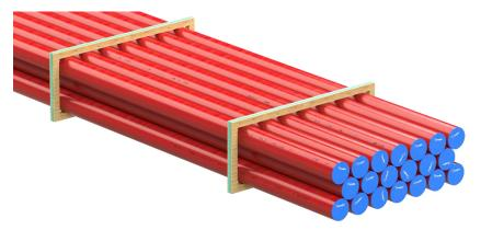
**EVOCAB STING** cable protection pipes are made of high-density polyethylene (HDPE) and designed for trenchless installations (e.g., horizontal directional drilling). These pipes have a smooth inner and outer surface and are available in pieces of various lengths and in rolls. Easy interconnection of pipes by using butt fusion method. Marking on the pipe includes length marks to determine installation length during trenchless installation process.
